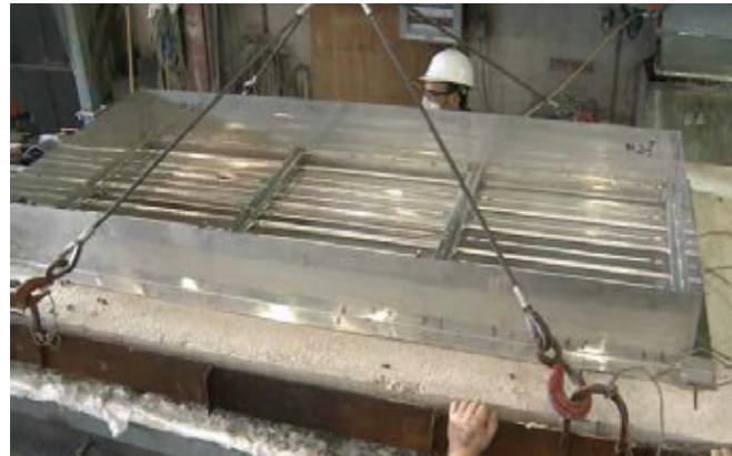
Damper test in fire
