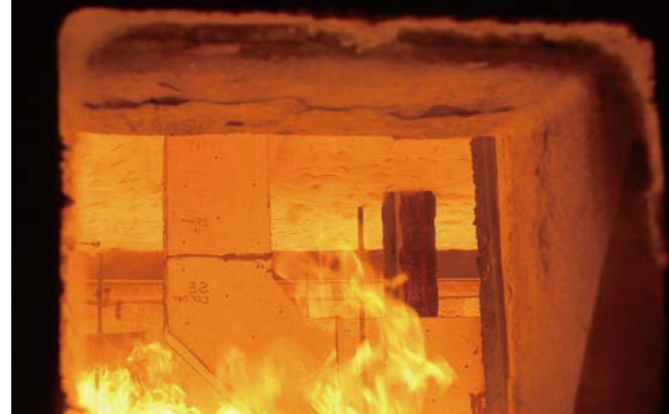
Cable tray test in fire
